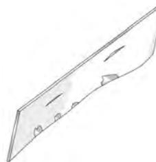
The photo shows a crack in a nickel blade, undetectable with the eye.
