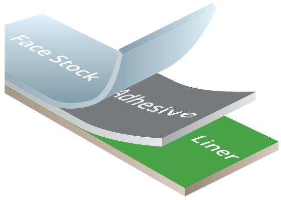
**Face Stock:** 2.4 mil topcoated gloss white polyimide film offering excellent chemical resistance combined with superior high heat resistance. The material will not curl and is designed to survive high teperatures of lead-free solder processes.
