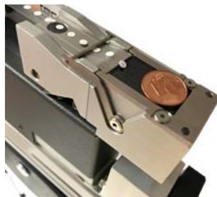
Apply of a round pressure compensation seal (PCS), 2mm diameter
